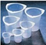
Transparent polypropylene beaker with three pouring lips for dripless dispensing.
